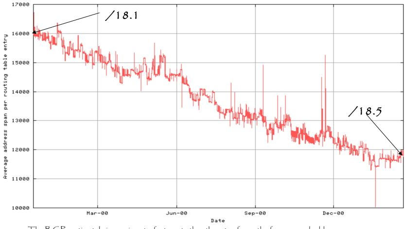
The BGP routing tale is growing at a faster rate than the rate of growth of announced address space
